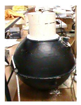
Figure 2 – The integrating photometer (at bottom: sphere in black colour) with the housing designed (cylinder in white colour) mounted on top, after February, 2019
